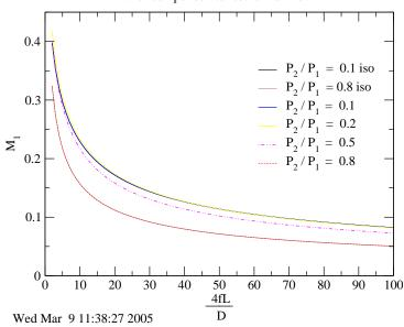
Fig. -10.23. The entrance Mach number as a function of dimensionless resistance and comparison with Isothermal Flow.
