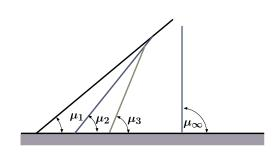
ber will be 1 and a normal shock will Fig. -14.8. The Mach waves that are supposed to occur, according the common explabe generated at zero inclination.
