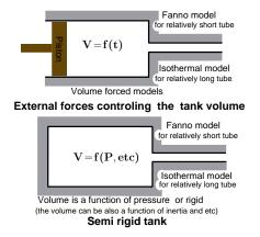
Fig. -12.1. The two different classifications of models that explain the filling or evacuating of a single chamber.
