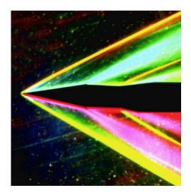
Fig. -14.11. Color-schlieren image of a two dimensional flow over a wedge. The total deflection angel (two sides) is  $20^\circ$  and upper and lower Mach angel are  $\sim 28^\circ$  and  $\sim 30^\circ$ , respectively. The image show the end–effects as it has thick (not sharp transition) compare to shock over a cone. The image was taken by Dr. Gary Settles at Gas Dynamics laboratory, Penn State University.
