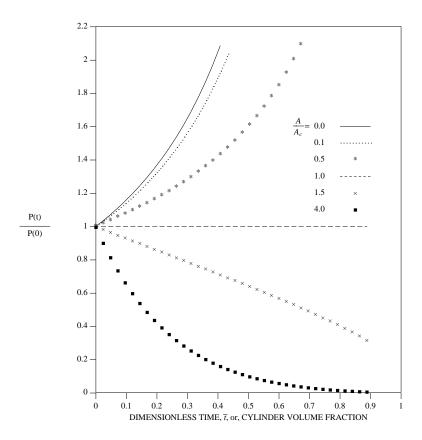
$\textit{Fig. -13.3.} \ \textit{The pressure ratio as a function of the dimensionless time for choked condition.}$
