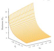
Fig. -6.23. Maximum Mach number that can be obtained for given specific heats.
