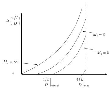
Fig. -10.16. The extra tube length as a function of the shock location,  $\frac{4 f L}{D}$  supersonic branch.
