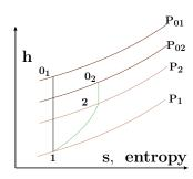
Fig. -7.3. Description to clarify the definition of diffuser efficiency.
