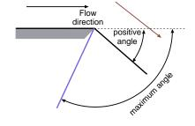
Fig. -15.1. The definition of the angle for the Prandtl–Meyer function.
