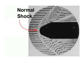
Fig. -14.4. Flow around spherically blunted  $30^{\circ}$  conecylinder with Mach number 2.0. It can be noticed that the normal shock, the strong shock, and the weak shock coexist.
