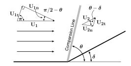
Fig. -14.3. A typical oblique shock schematic.
