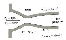
Fig. -7.2. A nozzle with normal shock.
