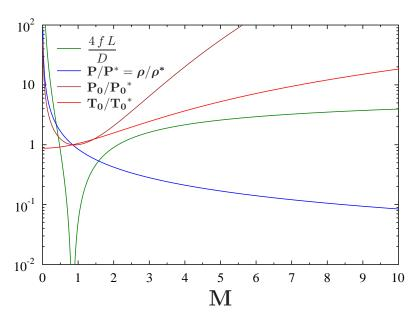
Fig. -9.2. Description of the pressure, temperature relationships as a function of the Mach number for isothermal flow.
