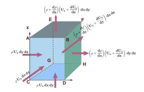
Fig. -3.5. The mass balance on the infinitesimal control volume.
