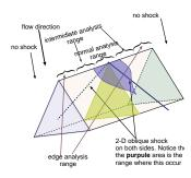
Fig. -14.12. Schematic of finite wedge with zero angle of attack. Notice that the purple area is only range where standard oblique shock analysis is applied.
