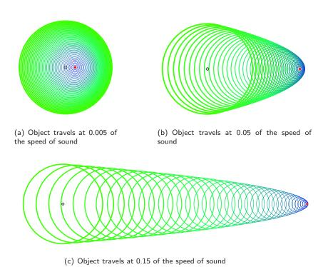
Fig. -4.5. Moving object at three relative velocities. The gray point in the first circle is the initial point the object. The finial point is marked by red circled with gray filled. Notice that the circle line thickness is increase with the time i.e the more green wider circle line thickness. The transition from the blue fresher lines to the green older lines is properly marked.
