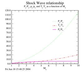
Fig. -6.4. The ratios of the static properties of the two sides of the shock.
