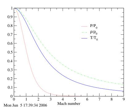
Fig. -5.3. The stagnation properties as a function of the Mach number,  $k=1.4\,$
