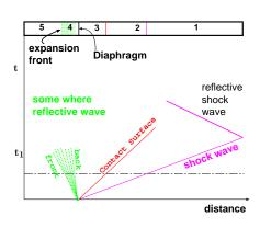
Fig. -6.22. The shock tube schematic with a pressure "diagram."
