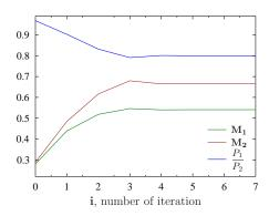
Fig. -10.20. Conversion of solution for given  $\frac{4 f L}{D} = 0.5$  and pressure ratio equal 0.8.
