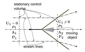
Fig. -14.25. The diagram that explains the shock drag effects of a moving shock considering the oblique shock effects.
