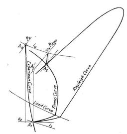
Fig. 51.—"Condition loci" for compression shock
