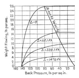
searchers were the first ones Fig. -1.4. Flow rate as a function of the back pressure taken to realized that choking can after Stodola 1927 Steam and Gas Turbines occurs at different Mach number  $(1/\sqrt{k})$  other than the isothermal pipe.
