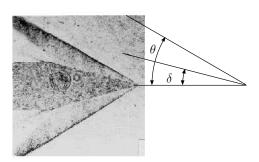
Fig. -14.17. Oblique shock occurs around a cone. This photo is courtesy of Dr. Grigory Toker, a Research Professor at Cuernavaco University of Mexico. According to his measurement, the cone half angle is  $15^{\circ}$  and the Mach number is 2.2.
