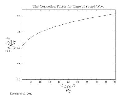
Fig. -4.4. The Correction Factor for Time of Sound Wave.
