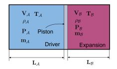
Fig. -6.27. Shock tube schematic for thermodynamics consideration at initial stage.
