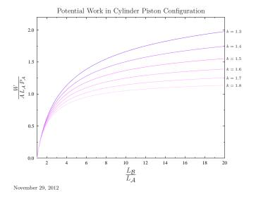
Fig. -2.2. Dimensionless work available in a cylinder piston configuration.
